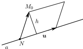
$$[\overline{NM}_0 \times \vec{u}] = \begin{vmatrix} \vec{i} & \vec{j} & \vec{k} \\ 0 & -4 & 8 \\ 2 & -1 & 3 \end{vmatrix} = (-4; 16; 8),$$
