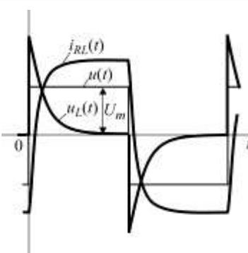
$i_{RL}(t) = \frac{U_m}{R} (1 - 2e^{-t/\tau})$ $u_R(t) = U_m (1 - 2e^{-t/\tau})$ $u_L(t) = 2U_m e^{-t/\tau}$ $\tau = \frac{L}{R}$ | $i_{RL}(0_+) = i_{RL}(0_-) = -\frac{U_m}{R};$ $i_{RL}(\infty) = \frac{U_m}{R}$ $u_R(0_+) = -U_m;$ $u_R(\infty) = u_R(0_-) = U_m$ $u_L(0_+) = 2U_m;$ $u_L(\infty) = u_L(0_-) = 0$ |
