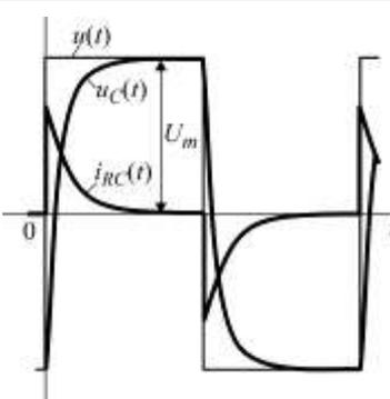
$i_{RC}(t) = \frac{2U_m}{R} e^{-t/\tau}$ $u_R(t) = 2U_m e^{-t/\tau}$ $u_C(t) = U_m (1 - 2e^{-t/\tau})$ $\tau = RC$                | $i_{RC}(0_+) = \frac{2U_m}{R};$ $i_{RC}(\infty) = i_{RC}(0_-) = 0$ $u_R(0_+) = 2U_m;$ $u_R(\infty) = u_R(0_-) = 0$ $u_C(0_+) = u_C(0_-) = -U_m;$ $u_C(\infty) = U_m$             |
