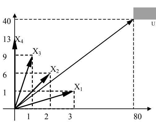
$$\begin{aligned} 3x_1 + 2x_2 + x_3 &\geq 80 \\ x_1 + 6x_2 + 9x_3 + 13x_4 &\geq 40 \end{aligned}$$
